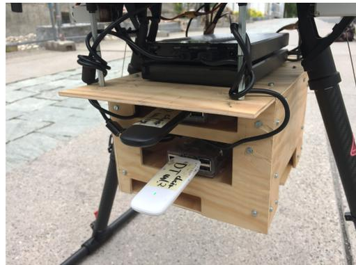
**(b)** Two of the four Raspberry Pi computers are visible, the other two are similarly attached on the opposite side of the wooden box. Two batteries that are fixed on top of the case power the single-board computers.
